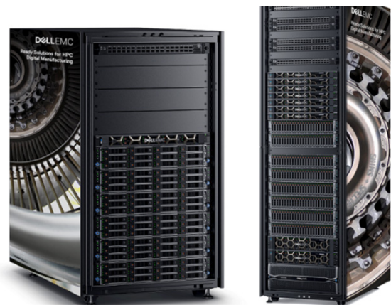
The HPC cluster appliance from TotalCAE, based on a Dell EMC PowerEdge system with Intel Xeon Gold processors, enables simulation as a service using engineering simulation applications.
